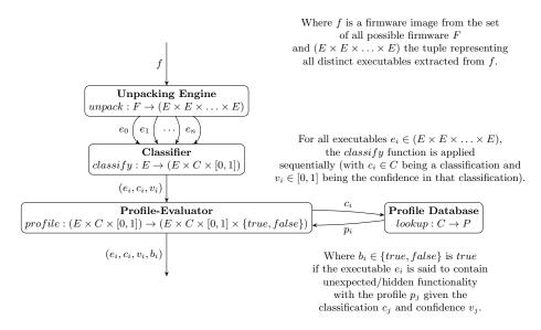
Fig. 1: HumIDIFy system architecture
